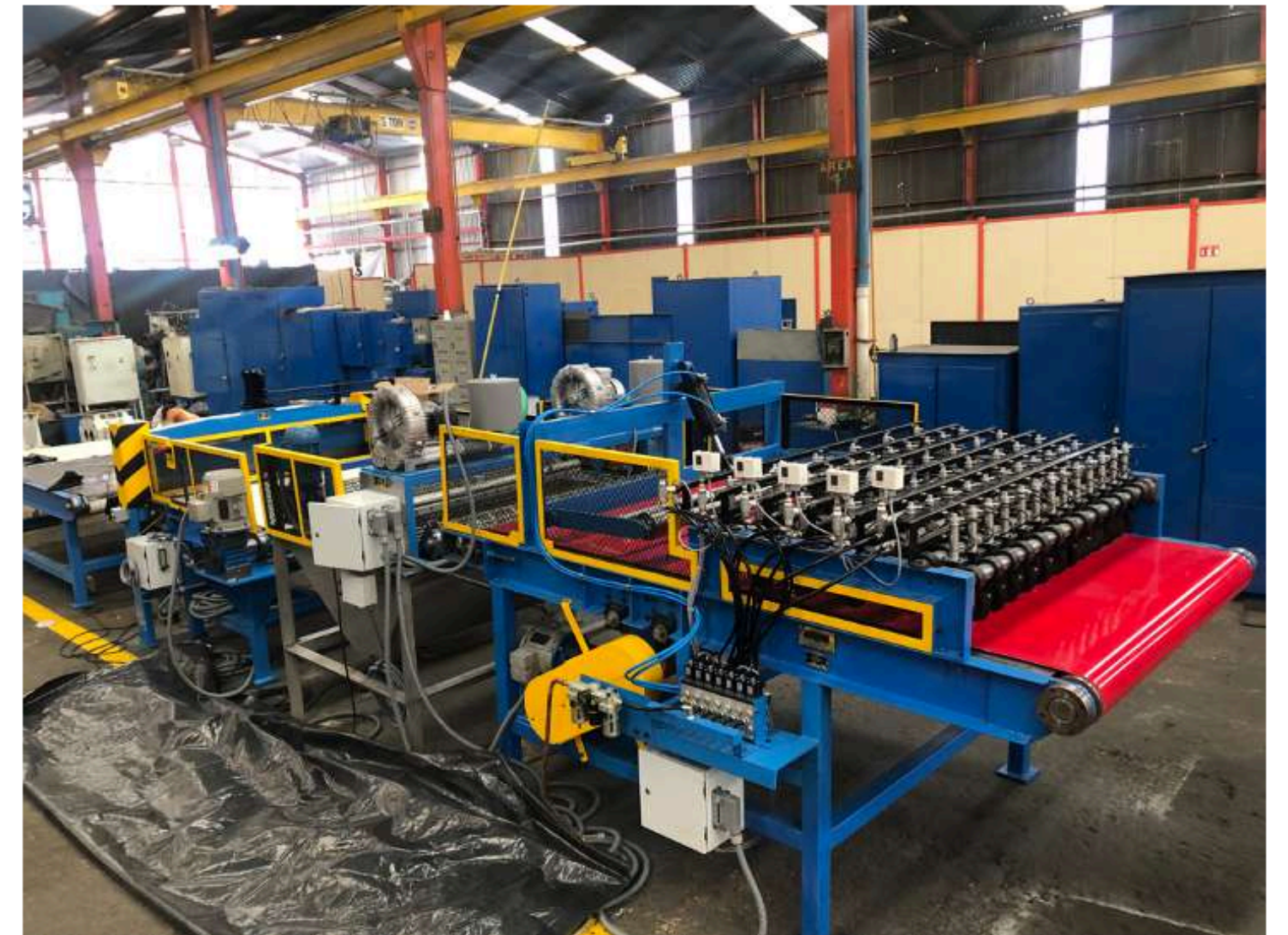
Custom multi-knife conveyor guillotine system
